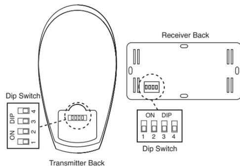
Figure 1 - Setting DIP Switches
