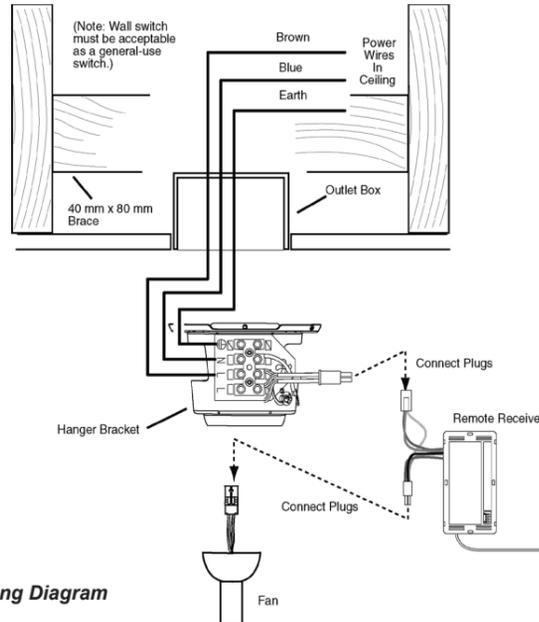
Figure 2 - Wiring Diagram
