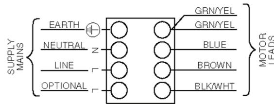
Figure 3 - Terminal Block Connections
