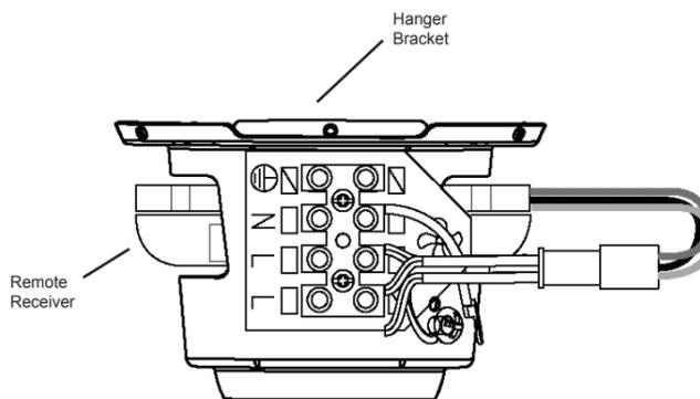
Figure 4 - Remote Receiver in Hanger Bracket
